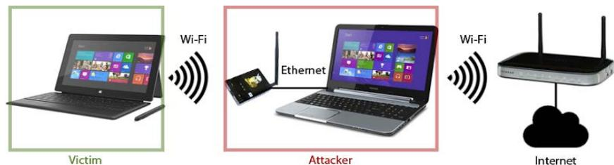
Figure 3. Fake access point - Man-in-the-middle attack (MITM)
