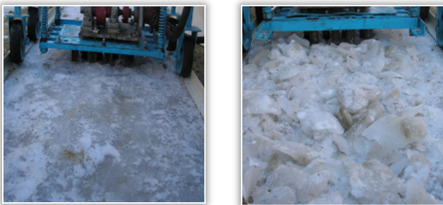
Figure 2 - Laboratory installation for the research of wedge-shaped destructive elements placed on the shocking plate: 1 – a frame of working body. 2 – the indents of the first row. 3 – the indents of the second row.
