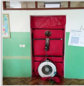
Figure 1 - Measurement of airtightness in classroom with Minneapolis Blower Door equipment and detection of typical air leakage places
