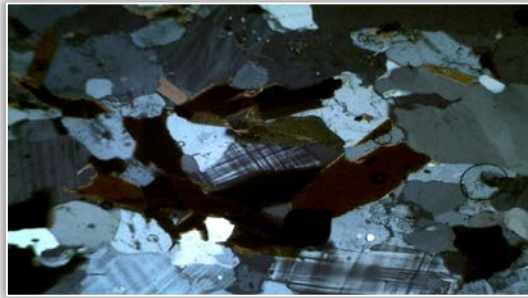
Plate A 3 : Photomicrograph of the Sample of granite under cross Polar
