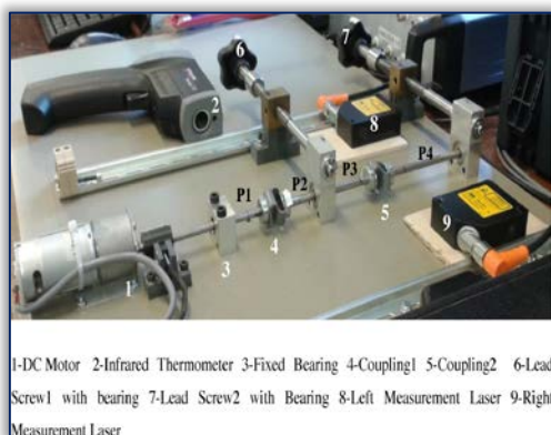
Figure 5. Test-rig for temperature monitoring [15]
