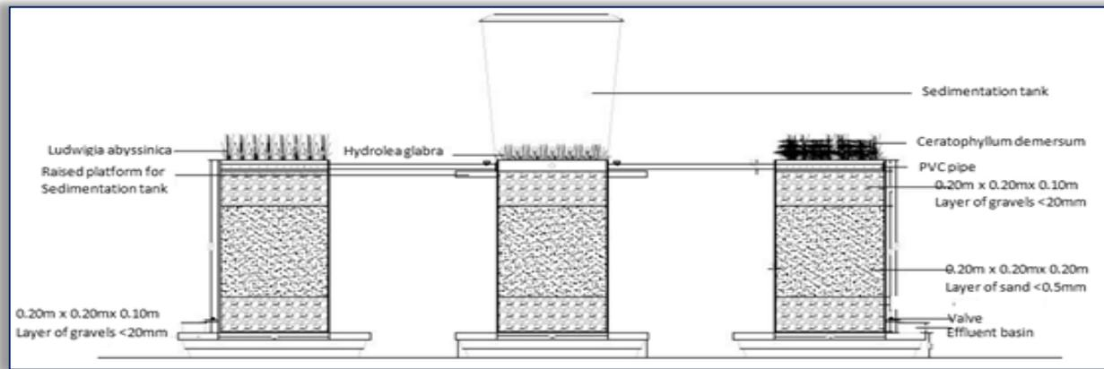
Figure 2: Schematic diagram of Constructed Wetland Design
