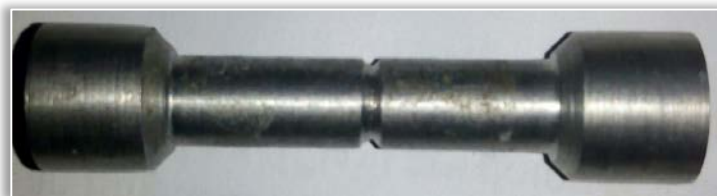
Figure 12: Circumferential Notch Tensile (CNT) specimen
