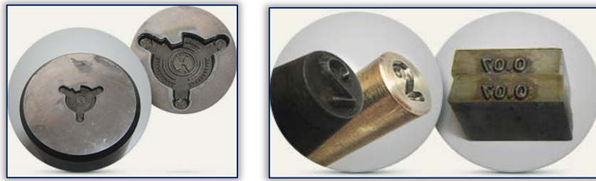
Figure 8-Examples of machined parts with ECM made from tool steels [9]
