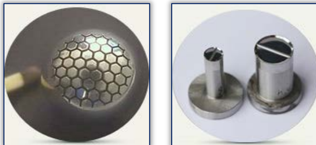
Figure 6-Examples of machined parts with ECM made from high-carbon chromium steels [9]
