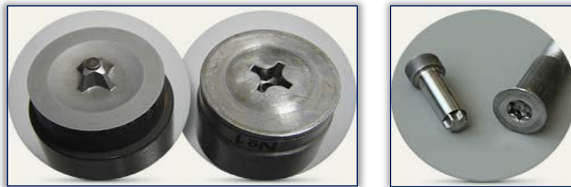
Figure 10 -Examples of machined parts with ECM made from High Strength Steels [9]
