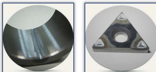
Figure 13-Examples of machined parts with ECM made from ceramic-metal hard alloys (WC-Co, WC-TiC-Co) [9]
