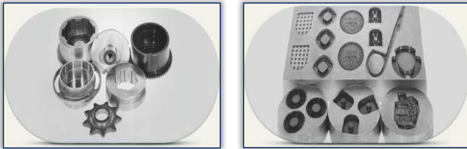
Figure 4-Examples of machined parts with ECM made from alloy steels and construction steels [9]
