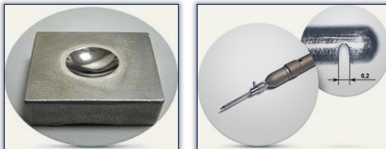
Figure 7-Examples of machined parts with ECM made from stainless chrome-nickel steels [9]
