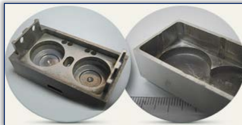
Figure 11- Examples of machined parts with ECM made from nickel alloys [9]
