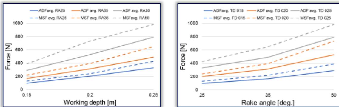
Figure 4 – Variation of draft force and starting force with working depth and rake angle of the tool.
