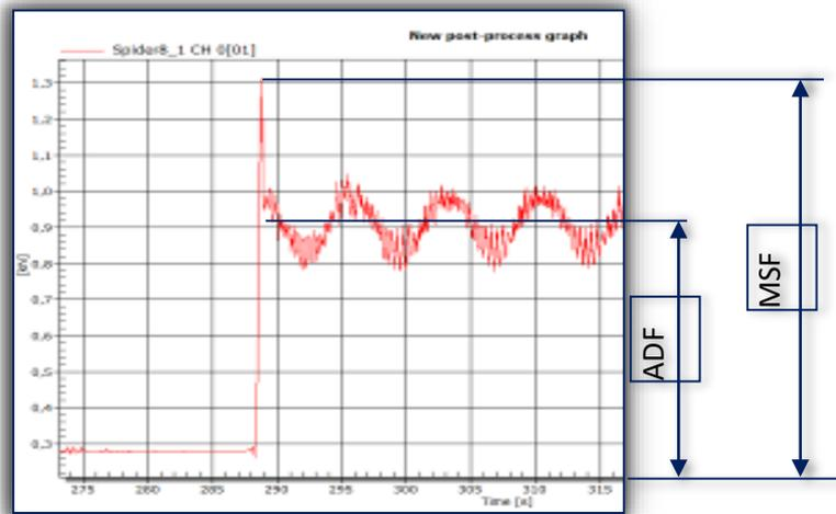
Figure 3 – Catman Easy print screen of recorded data during the starting phase. ADF – Average Draft Force, MSF – Maximum Starting Force.
