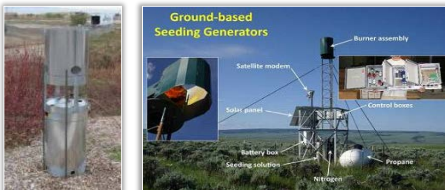
Figure 13 – Ground-based generator (propane burner) [18,19]
