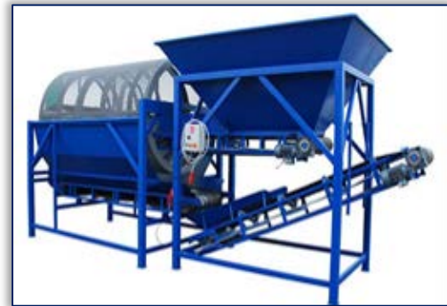
Figure 7 - OPTION rotary sieve installation for separating grape seed from marc, Italy [9]
