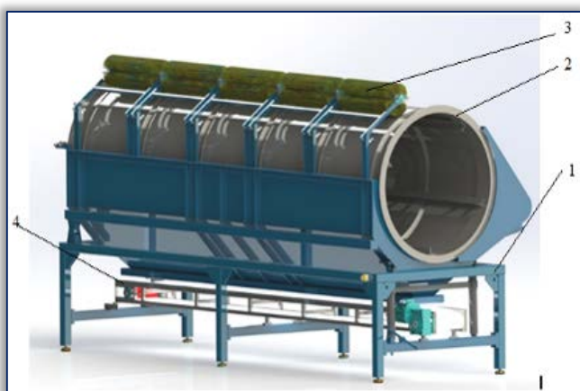
Figure 5 - Onmak Makina grape seed separator, Turchi [21] 1 - Metallic frame; 2 - Rotary cylindrical sieve; 3 - exterior rotary brush; 4 - rubber belt conveyor
