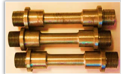
Figure 3. Sample for determining the hot deformability by torsion [10]
