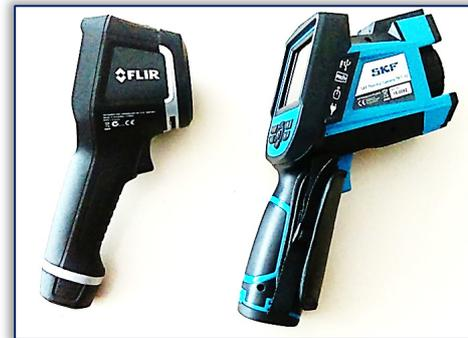
Figure 4. Thermal cameras: FLIR (left) and SKF (right)
