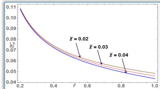
Figure 4: Radial Stress  $\bar{\sigma}_{rr}$  along  $\bar{r}$ -direction for different values of  $\bar{z}$
