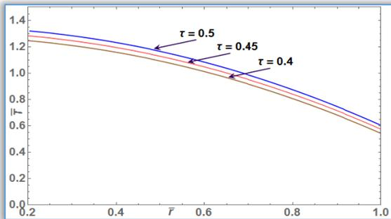
Figure 1: Temperature distribution along  $\bar{r}$ -direction for different values of time
