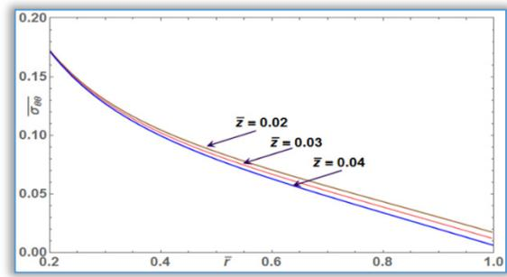
Figure 6: Tangential Stress  $\bar{\sigma}_{\theta\theta}$  along  $\bar{r}$ -direction for different values of  $\bar{z}$
