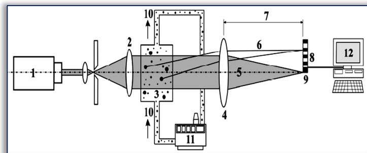
Figure 4 - General view of the laser diffraction device
