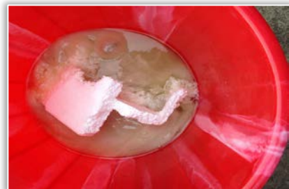
Figure 4: Polystyrene dissolved in petrol and kept for four days
