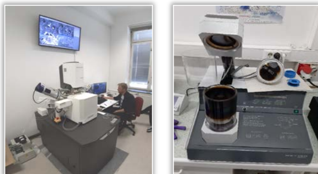
a) Figure 3. Scanning electron microscopy (a); Sputter Coater Balzers SCD 050 (b)
