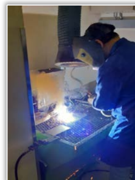
a) Figure 2. Sampling in case of welding process with use a suction device (a), and without use a suction device (b)
