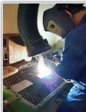
a) Figure 2. Sampling in case of welding process with use a suction device (a), and without use a suction device (b)
