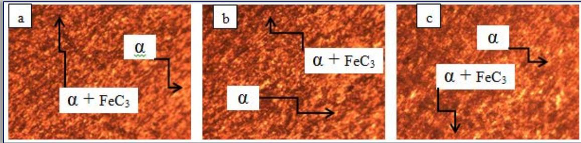
Plate 2. Micrograph of the (a) weldment; (b) HAZ; (c) base metal of 45° bevel angle after etched in 2% Nital solution at magnification 100x
