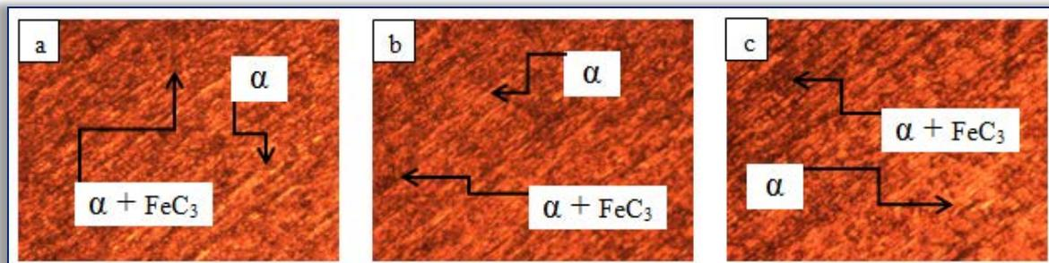
Plate 4. Micrograph of the (a) weldment; (b) HAZ; (c) base metal of 90° bevel angle after etched in 2% Nital solution at magnification 100x
