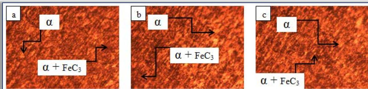
Plate 1. Micrograph of the (a) weldment; (b) HAZ; (c) base metal of 30° bevel angle after etched in 2% Nital solution at magnification 100x
