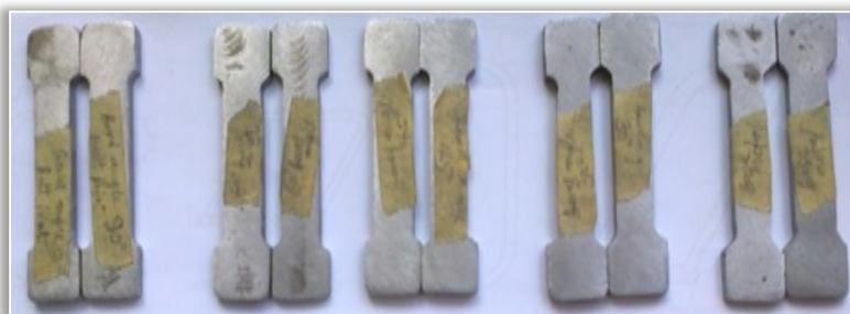
Figure 2: Machined (milled) tensile and microstructures tests samples
