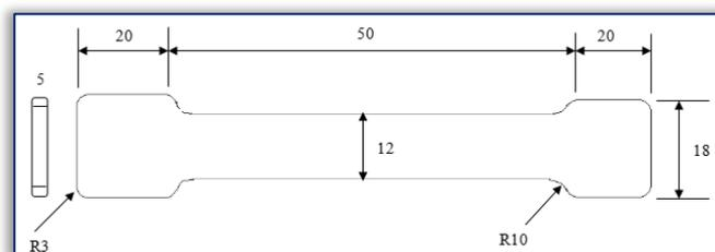
Figure 1: Tensile Strength Sample Schematic Drawing
