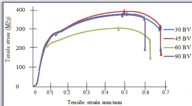
Figure 3: Variation of Tensile Stress for Welded Samples at Different Bevel Angles
