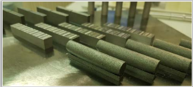
Figure 4. Pieces on the tray after additive manufacturing
