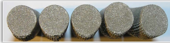
Figure 6. Pieces manufactured in laid position from top view. It can be seen well that those are deflected
