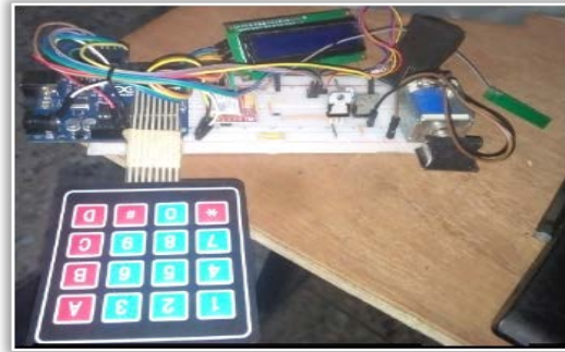
Figure 4b: Designed project on a bread board with the keypad for registration of fingerprint
