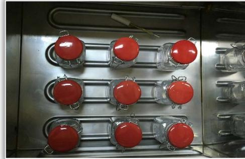
Figure 4. The heating furnace and containers with three samples of each type of magnesium alloy placed in the heating furnace
