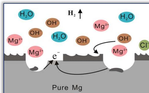
Figure 1. Schematic representation of the pure Mg corrosion
