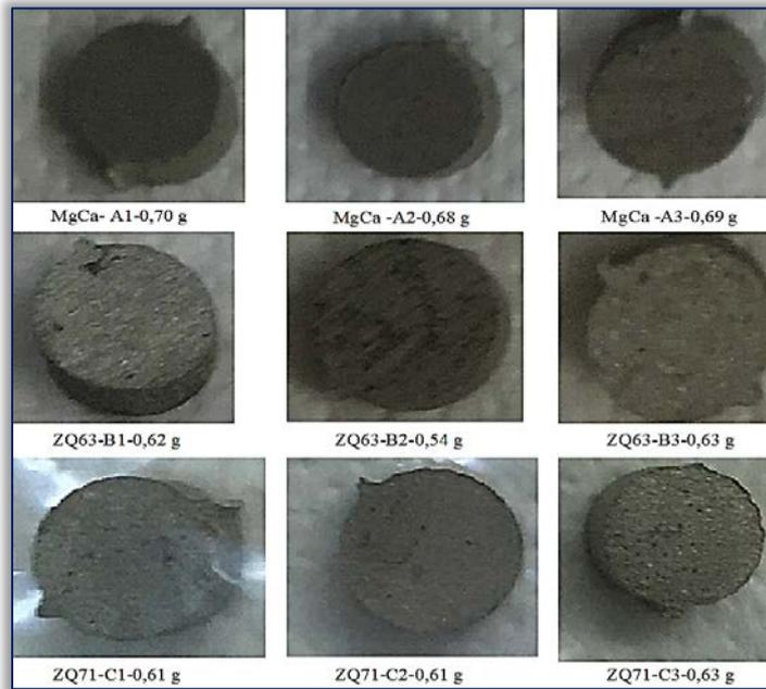
Figure 5. Samples from each type of magnesium alloy before immersion
