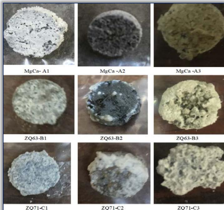
Figure 6. Samples from each type of magnesium alloy after immersion
