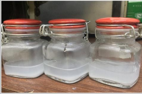
Figure 3. Containers with Ringer's solution to simulate human physiological fluids
