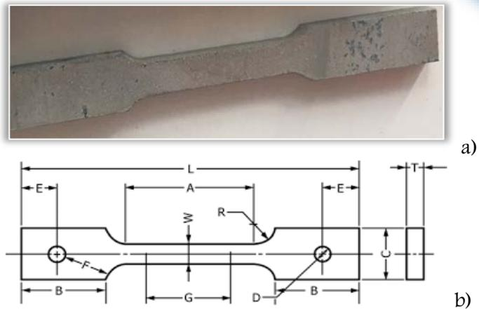
Figure 1. Rectangular Tension Test Specimens
