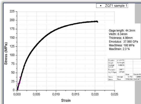
Figure 3. Stress–strain curve for ZQ71 alloys
