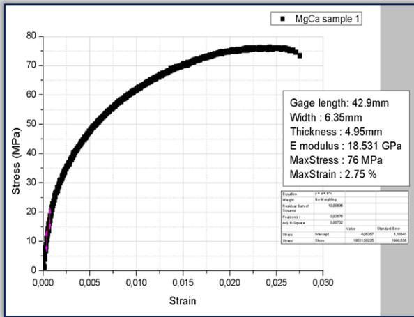
Figure 4. Stress-strain curve for MgCa alloys
