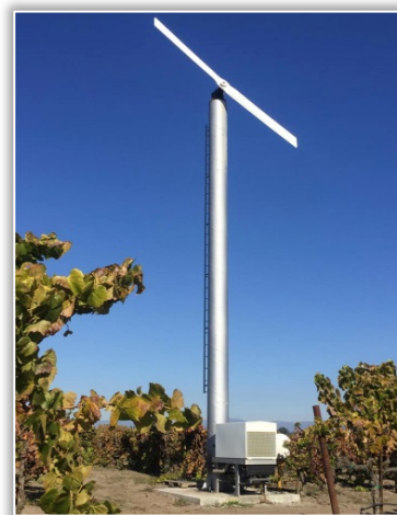
Figure 4. WIND MACHINE tower set up for orchards
