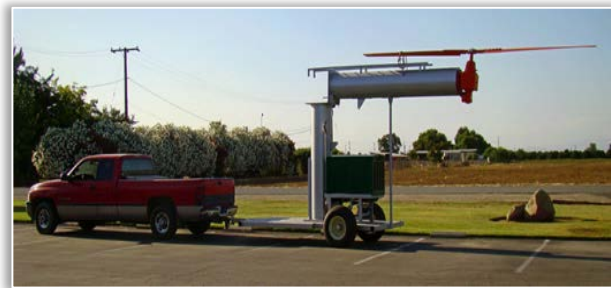
Figure 6. The mobile model of the ventilation tower for orchards WIND MACHINE
