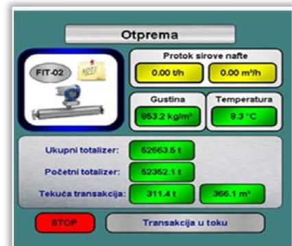
Figure 12. SCADA screen for flow meters
