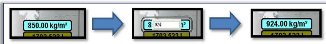
Figure 5. SCADA screen for manual input density in the tank
