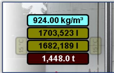
Figure 6. Density display, actual calculated sign, volume, reduced volume, calculated mass
