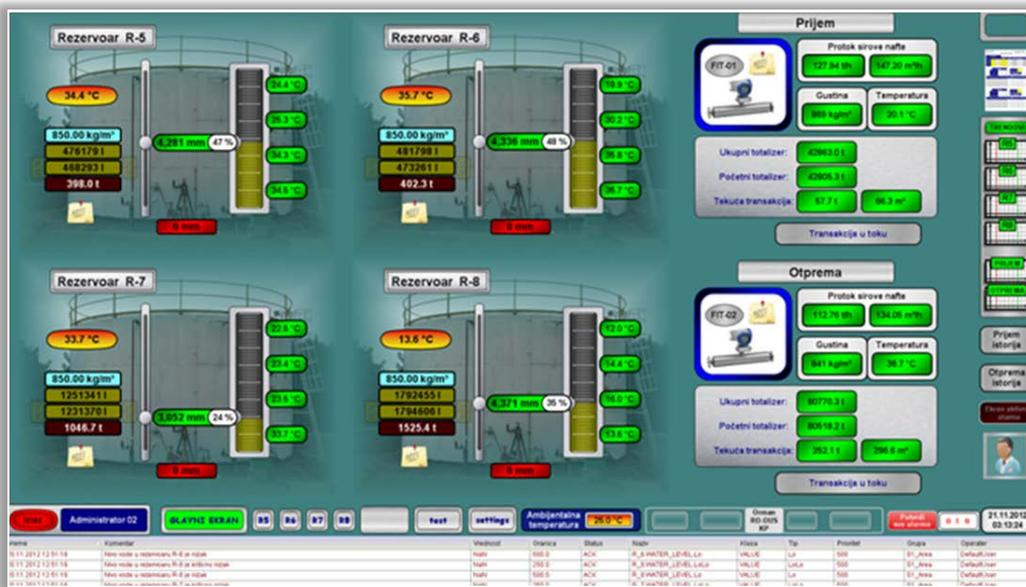
Figure 2. Main screen of SCADA application
