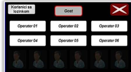
When logging is necessary to first select the user and then in the field below enter the password. Then ENTER is pressed and if the password matches the selected user, an “X” button will appear in the upper right corner. Pressing this button opens the SCADA system home screen as shown in Fig. 2.
