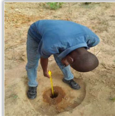
Figure 6. Measurement of water level drop
