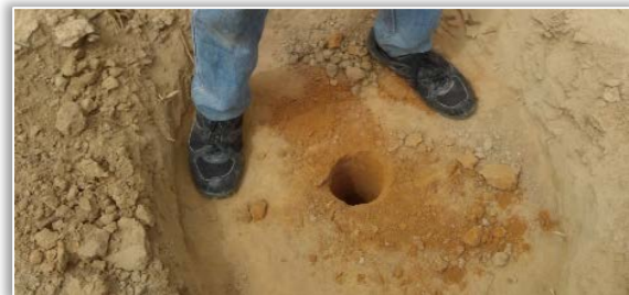
Figure 4. Porchet test cavity
