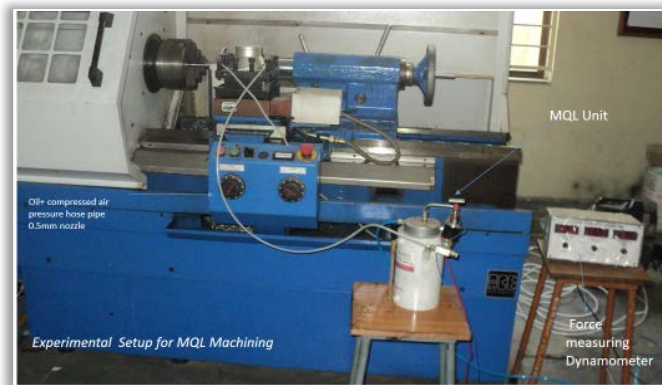
Figure 1. Experimental setup of MQL Machining
