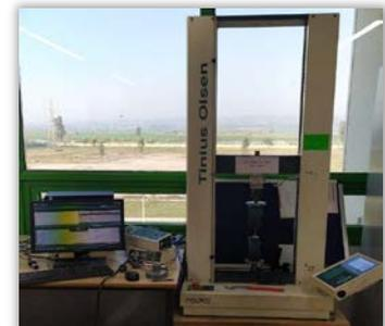
Figure 4: Tensile testing machine
