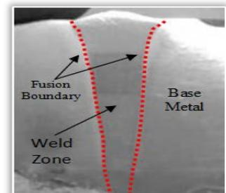
Figure 7: Macrostructure of weld joint
