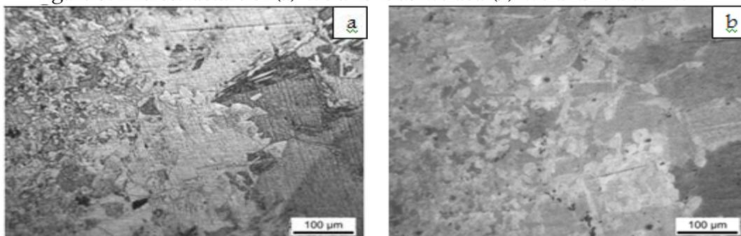
Figure 10: Microstructure of (a) fusion zone as-welded (b) fusion zone after PWHT
