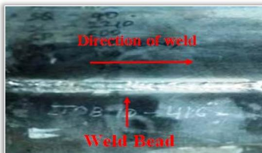
Figure 1: Fabricated AISI 409 joint with electron beam process
