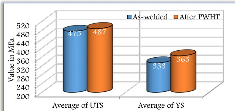
Figure 12: Average ultimate tensile strength and yield strength of as welded and after PWHT specimens
