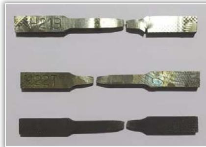
Figure 3: Extracted specimen for tensile testing before and after testing
