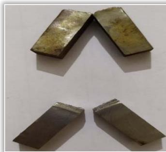
Figure 5: Extracted specimen before and after impact test
