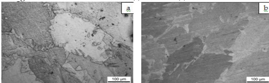
Figure 9: Microstructure of (a) Weld zone as-welded (b) Weld zone after PWHT
