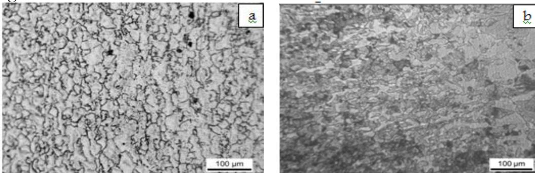
Figure 8 : Microstructure of AISI 409 (a) Base metal (b) Base metal after PWHT
