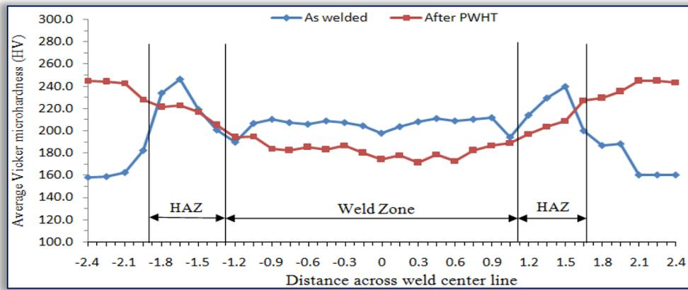
Figure 11: Average value of microhardness across the weld bead
