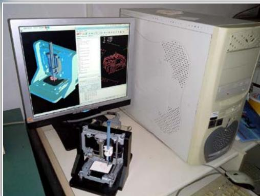
Figure 12. Machine work environment with PC control system and integrated virtual machine in the background
