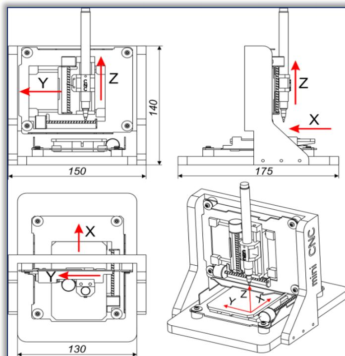
Figure 3. Drawing views of the complete assembly
