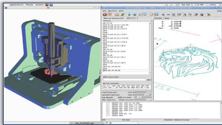
Figure 9. The Virtual machine integrated with the graphic user interface AXIS
