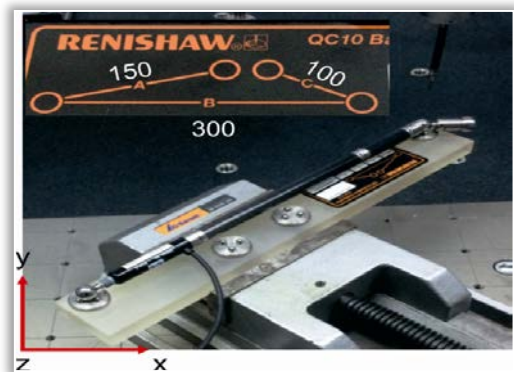
Figure 1. Reference gauge and ball bar fixed in fixture
