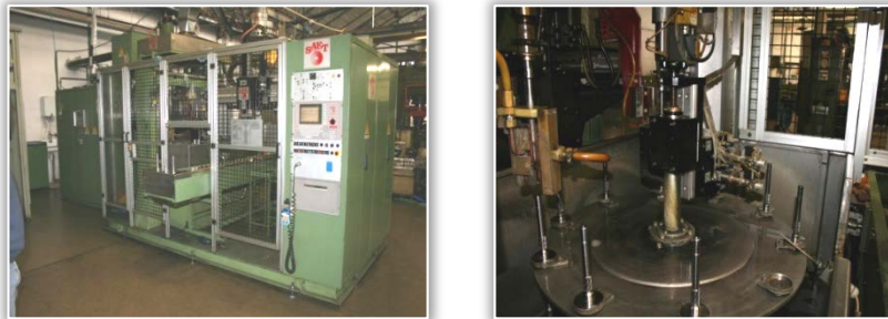
Figure 2. The spin case-hardening device 3KTC (left). Inductor and manipulation system (right). Heat treatment and device parameters are: theoretical power 93 kW, actual power 72,8 kW, Frequency 83 kHz, voltage 508 V, heating time 2.5 s, quenching time 1.5 s, and total time of life cycle 15 s.
