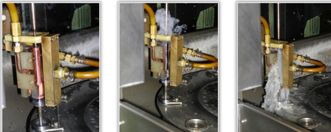
Figure 3. Chronological review of induction case-hardening process.
