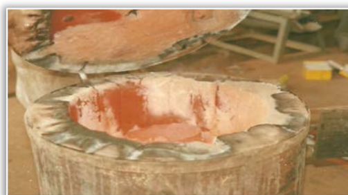
Figure 4. Evacuation of the furnace ash and unburnt briquettes
