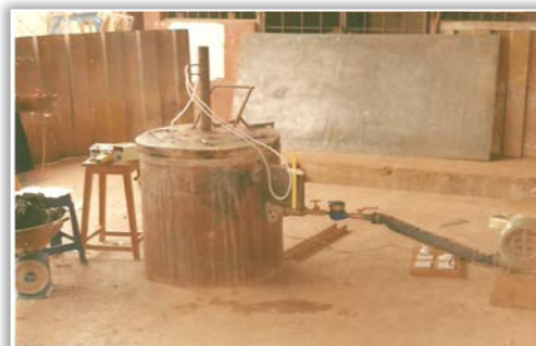
Figure 1. The furnace being fired with palm kernel shell briquettes
