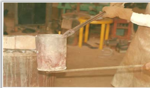
Figure 2. An opened non-ferrous melting furnace fired with palm kernel shell briquette when aluminum attained its pouring temperature
