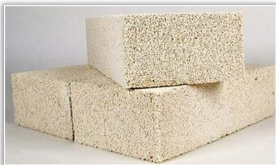
Figure 11. Ceramic blocks without refractory waste in the manufacturing recipe
