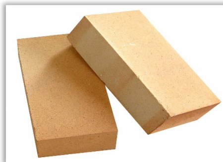
Figure 12. Ceramic blocks obtained using refractory waste in the manufacturing recipe
