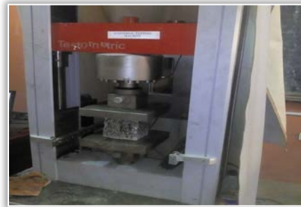
Figure 3: Curing process of cube specimen Figure 4: Process of testing cube specimen
