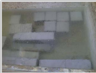
Figure 3: Curing process of cube specimen Figure 4: Process of testing cube specimen
