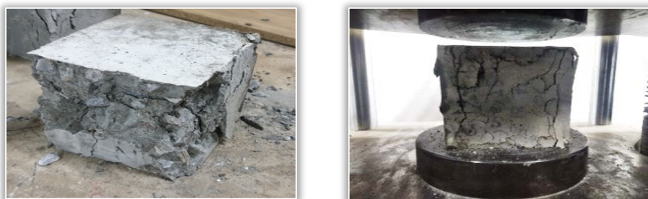
Figure 4. Specimen after compression failure (a) Plain Concrete (b) GFRC (0.2%)
