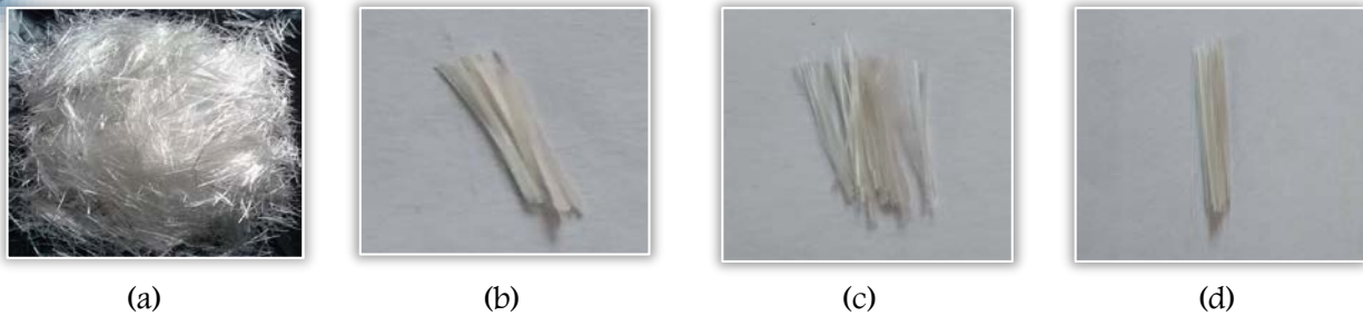
Figure 1. (a) Raw Glass Fiber (b) Glass Fiber (15 mm) (c) Glass Fiber (20 mm) (d) Glass Fiber (25 mm)
