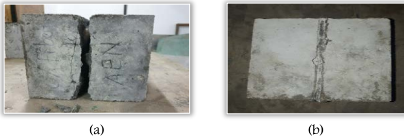
Figure 6. Specimen after tension failure (a) Plain Concrete (b) GFRC (0.2%)
