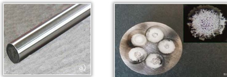
Figure 1. Representative image of the a) bar batch b) specimen sparked 5 times
