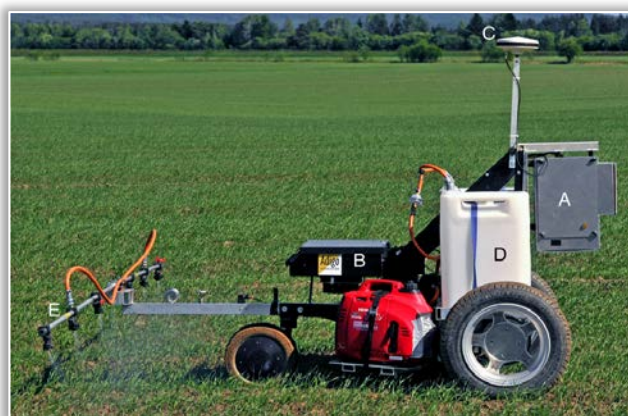
Figure 7. Robot – that acquires images and processes them for the purpose of weed monitoring and spraying A = box with camera and xenon lighting; B = box with computer, GPS and memory disk; C = GPS antenna; D = herbicide tank; E = spraying ramp, [6]
