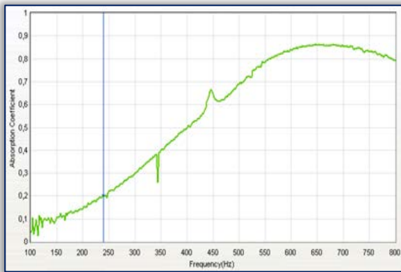
Figure 10. Display of the sound absorption coefficient for a two-layer material, composed of 2 cm thick recycled rubber positioned closer to the sound source and of 2 cm thick Ekomolitan positioned at the end in the frequency range of 100 to 800 Hz
