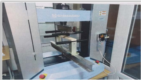
Figure 1. Bending of wood sample
