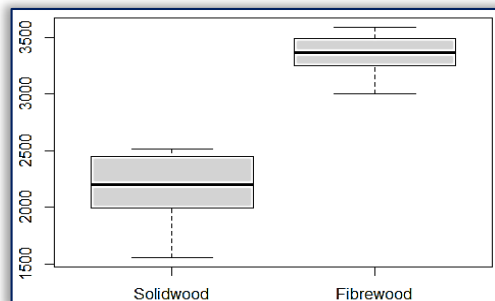
Figure 9. Box plots for the maximum force of solidwood (spruce) and fibrewood
