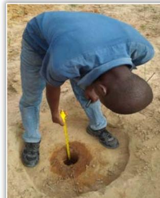
Figure 6- Measurement of water level drop
