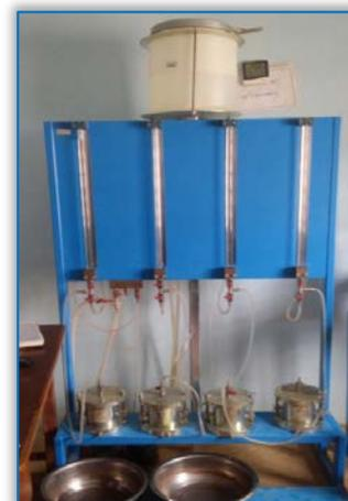
Figure 7- Principle scheme of variable load permeameter [10]      Figure 1- Constant or variable load permeameter
