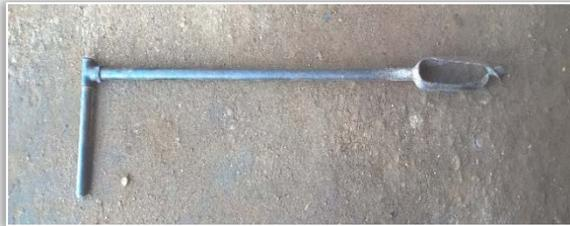
Figure 3- Manual auger
