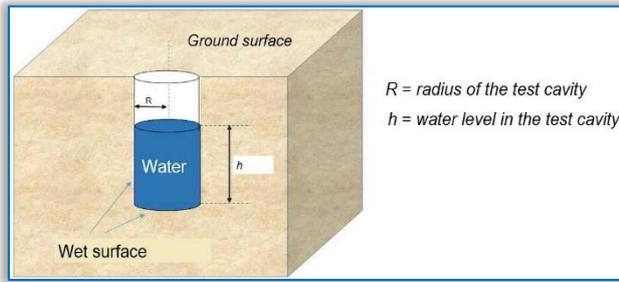
Figure 2- Principle schema of Porchet test [8]
