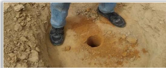
Figure 4- Porchet test cavity
