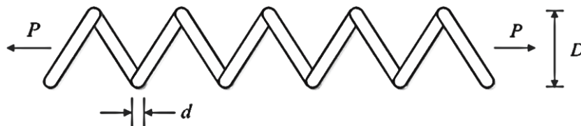
Figure 2. Tension/compression spring schematic 2D representation [9,10]
