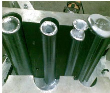
Fig. 2 Extraction of vibrated samples from the mold
