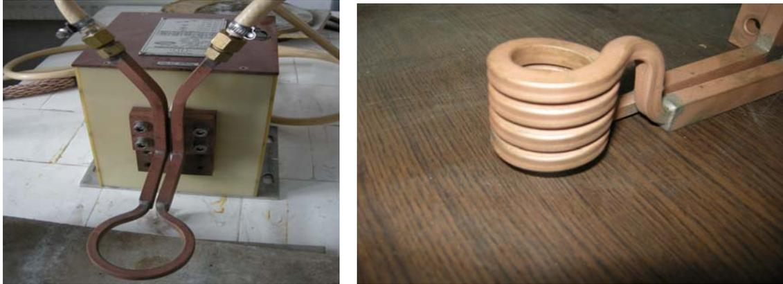
Fig.6 . Tempering transformer and inductor
