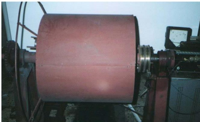
Figure 1. Rotary furnace for direct reduction
