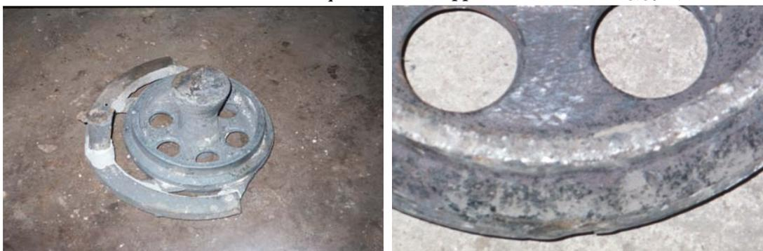
Figure 4. Casting presenting micro-cavities and pores.
