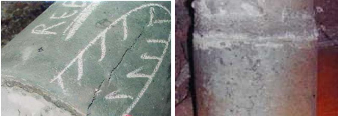
Figure 5. Castings presenting fissures.
