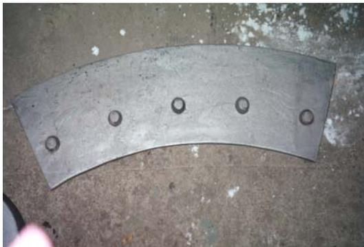
Figure 4. The metal model of casting *Armor*
