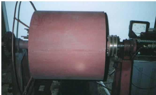
Figure 1. Rotary furnace for direct reduction
