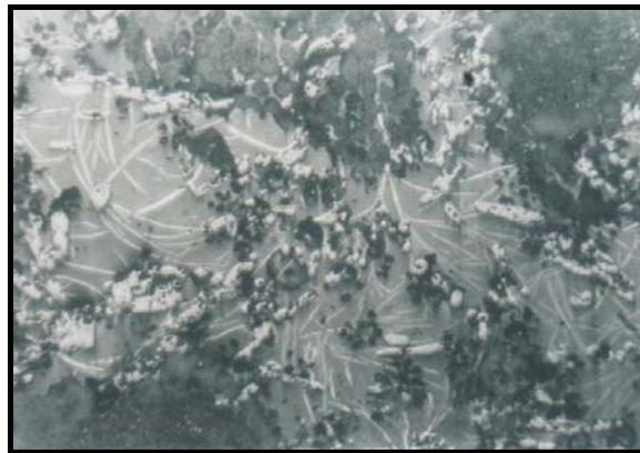
Fig. 1.10. Sample appeal  $FeCl_3+HCl$  chemical mass-R1 ceramic impregnated with Cu, marginal zone; 250X
