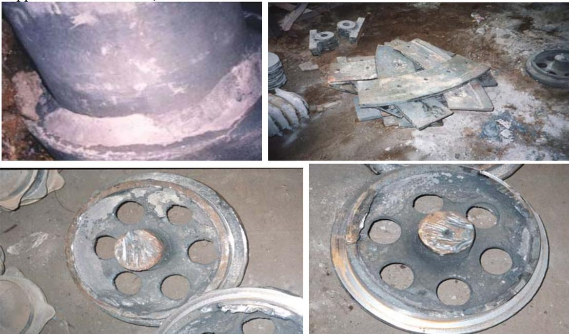
Figure 3. Castings presenting non-metallic inclusions and adherences. Cavities, micro-cavities and pores (B 311) appeared at a rate of 3,59%;
