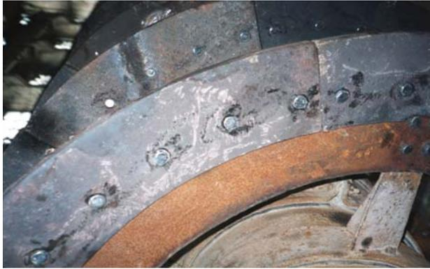
Figure 10. The armor mounted on spiral classifier
