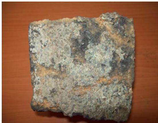
Fig.2. Interface between slag layer and brick
