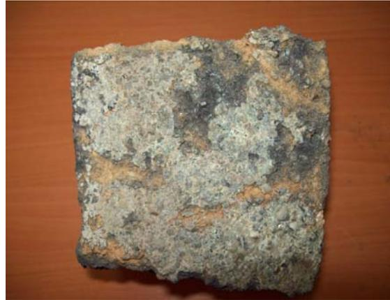
Fig.2. Interface between slag layer and brick
