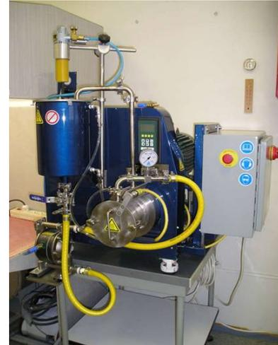
Figure 1. Horizontal high efficient attritor mill
