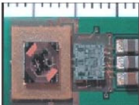
PICTURE 9. MICROSCOPIC DETAIL OF THE SENSOR PART. YOU CAN SEE THE LARGE OCTAGONAL EXCITATION COIL, WHICH IS ABOUT 3.8 mm ACROSS. THE FOUR SMALLER SENSING COILS BELOW IT ARE FAINTLY VISIBLE [13]
