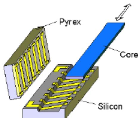
PICTURE 7. STRUCTURE OF THE MICRO COIL [12]
