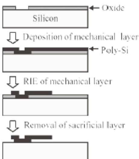
PICTURE 2. A BASIC SURFACE MICROMACHINING PROCESS
