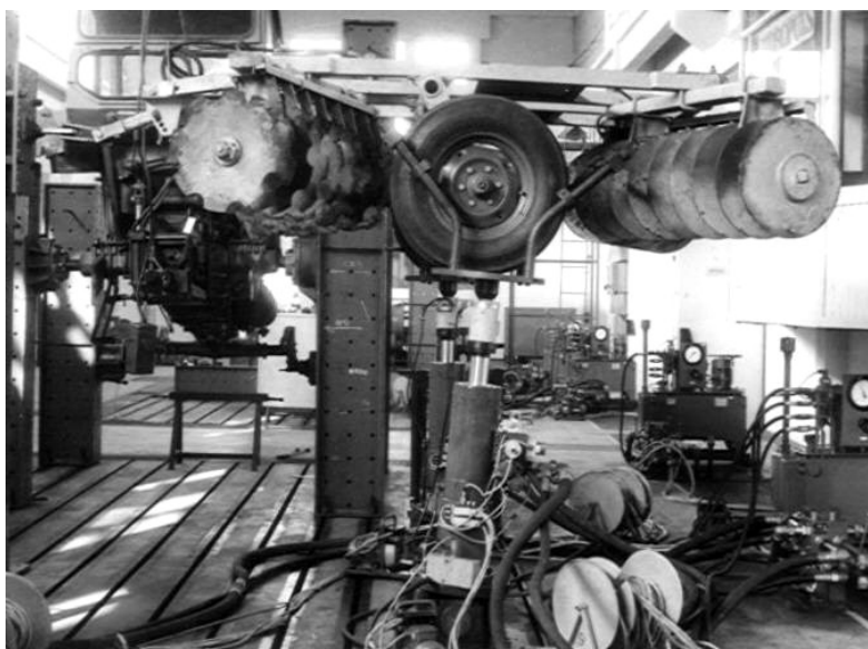
Figure 1- Simulated and accelerated test of the disk harrow GD 3.2, in the transport
