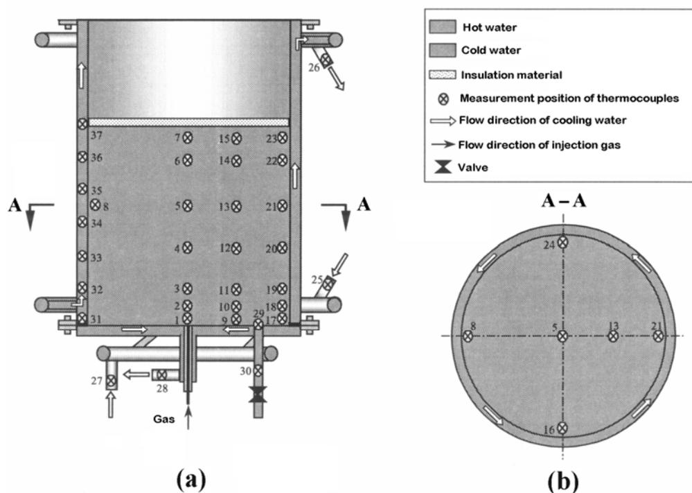
**Fig.1.** Hot-water model set-up.
