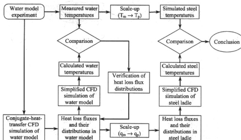
**Fig. 2.** Flow chart showing a method for verification of using hot-water model to simulate thermal stratification in steel ladles.
