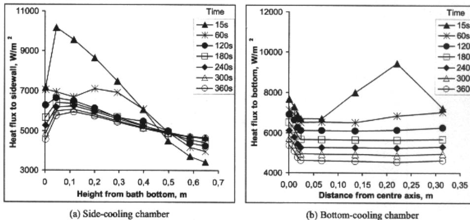
**Fig. 3.** Predicted distributions of heat fluxes from hot-water bath to cooling chambers.
