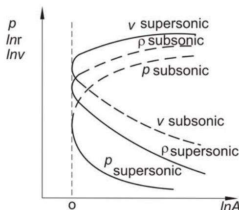
Figure 5. Changes of flow parameters during supersonic-subsonic transition depending on nozzle geometry change
