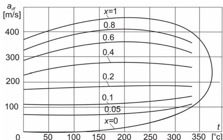
Figure 3. Dependence sound velocity on dryness rate and temperature
