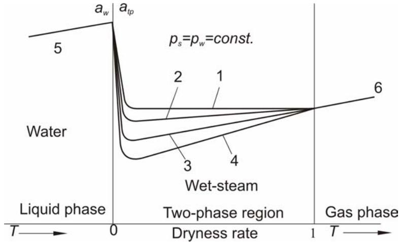
Figure 2. Change of sound velocity during isobaric transition from one phase to two phase region
