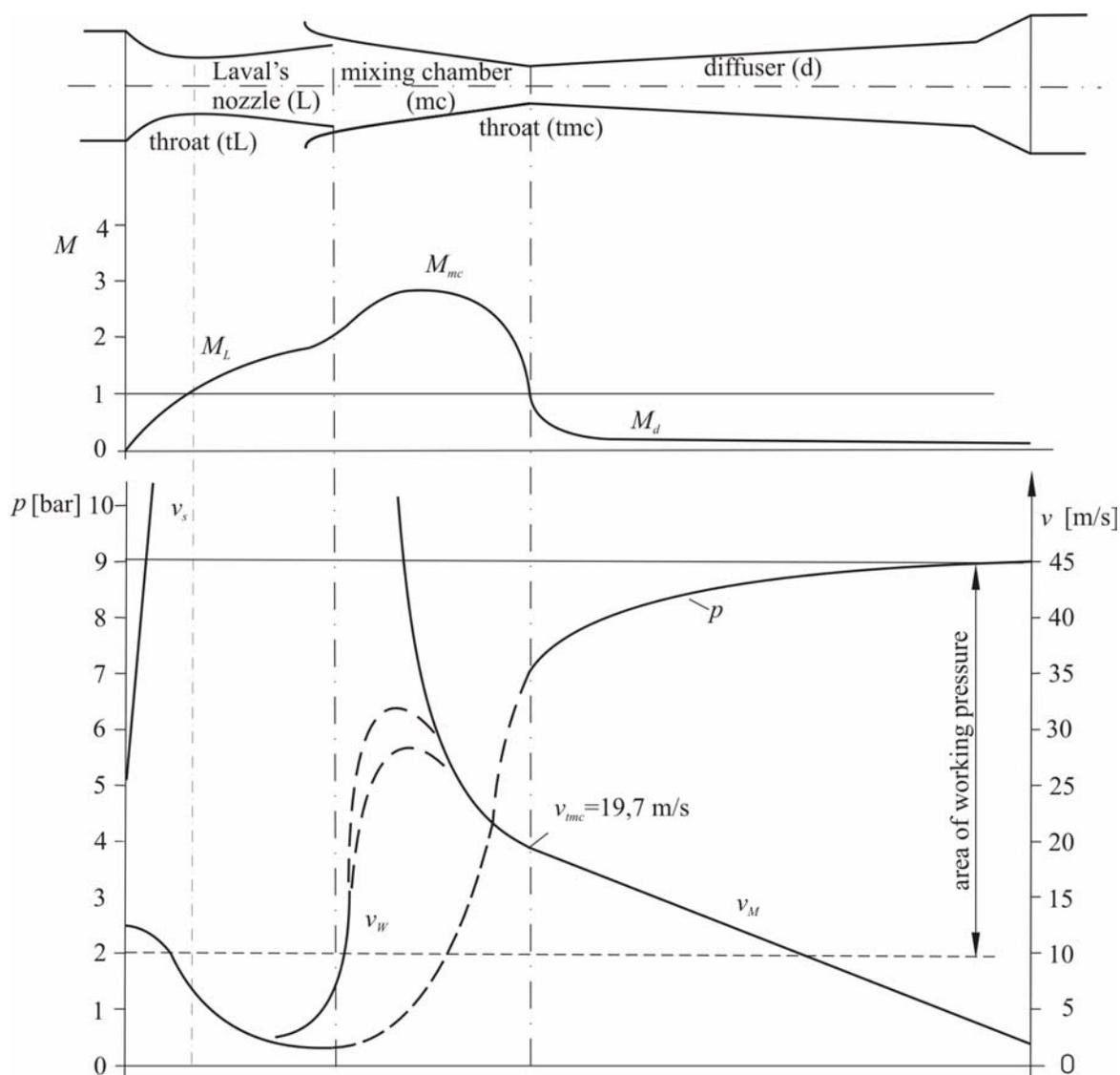
Figure 4. Diagrams of Mach number, pressure and mixture velocity in jet pump
