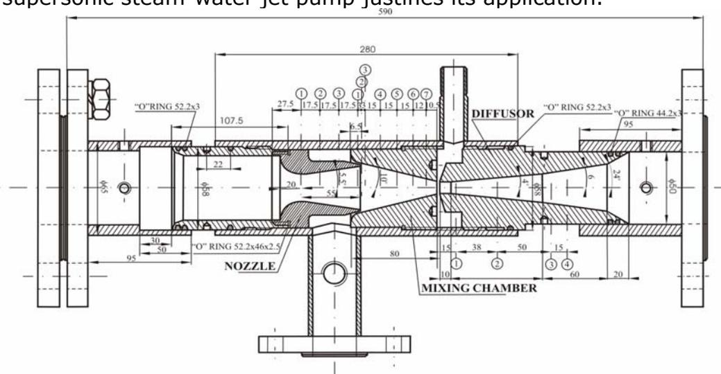
Figure 1. The outlook of steam-water jet pump
