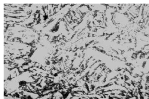
Figure 15. Sample 6.1-2 WELD [Nital etched 3%, x500]
