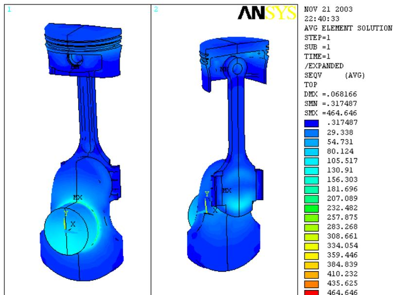
Figure 6: The equivalent stress field for the maximum rotative speed condition [MPa]
