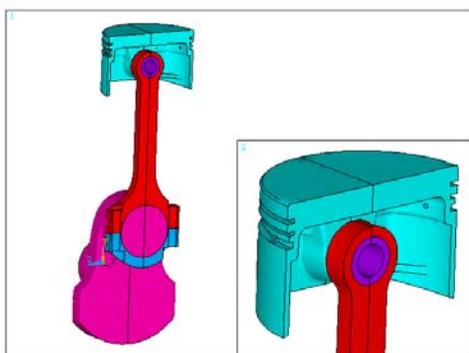
Figure 2: 3D model inserted in Ansys type finite elements
