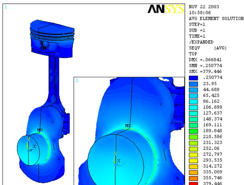
Figure 5: The equivalent stress field for the medium rotative speed condition [MPa]
