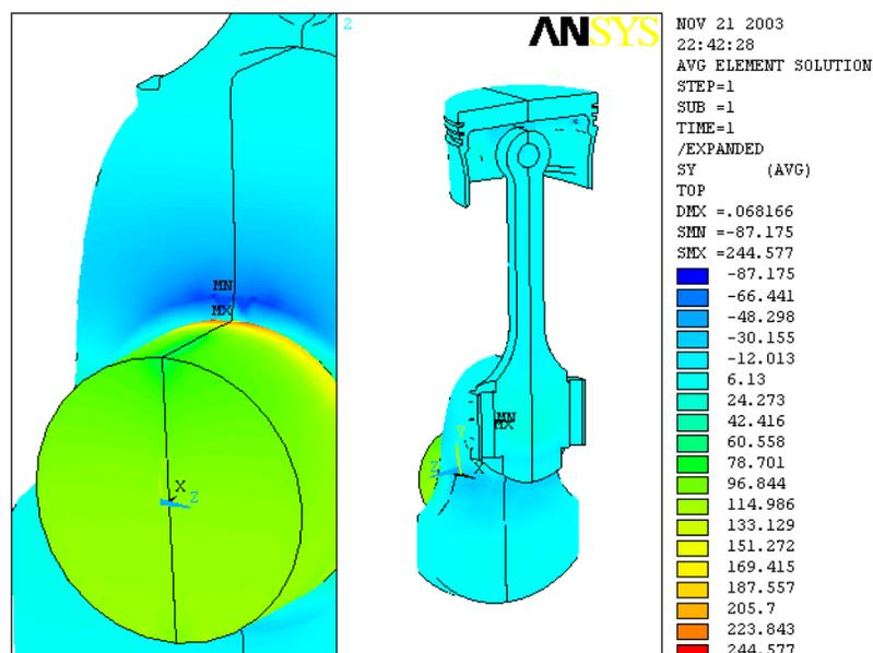
Figure 7: The stress field for the maximum rotative speed condition on the Oy axle [MPa]
