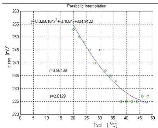
Fig. 2. The variation of the potential difference  $d_{eps}$  [mV] depending on the temperature of the NaCl solution, for a concentration of 1%.
