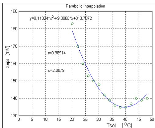
Fig. 16. The variation of the potential difference deps [mV] depending on the temperature of the NaCl solution, for a concentration of 15%.
