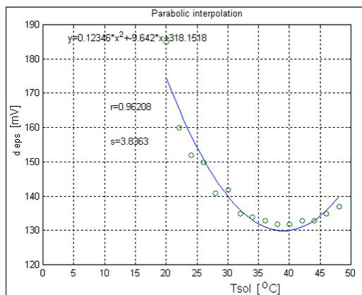
Fig. 7. The variation of the potential difference  $d_{eps}$  [mV] depending on the temperature of the NaCl solution, for a concentration of 6%.
