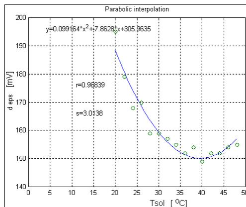
Fig. 6. The variation of the potential difference  $d_{eps}$  [mV] depending on the temperature of the NaCl solution, for a concentration of 5%.
