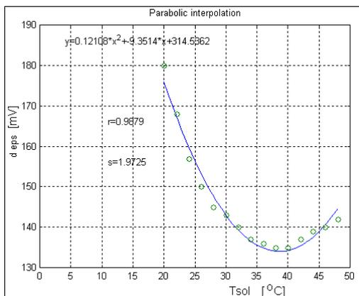
TABLE 2 - THE RESULTS OF THE CUBIC INTERPOLATION AT THE VARIATION OF THE ELECTROCHEMICAL POTENTIAL DIFFERENCES BETWEEN THE COATING AND THE METALLIC SUBSTRATE AND THE TEMPERATURE OF THE NaCl SOLUTION, FOR THE SAME CONCENTRATION.
