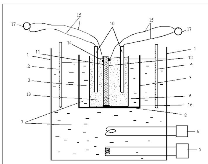
FIG. 1. THE ASSEMBLY MADE FOR THE DETERMINATION OF THE CORROSION RESISTANCE.
