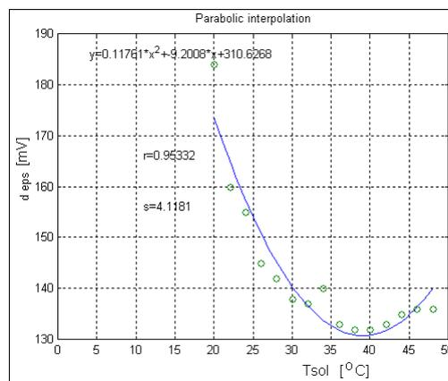
Fig. 11. The variation of the potential difference  $d_{eps}$  [mV] depending on the temperature of the NaCl solution, for a concentration of 10%.
