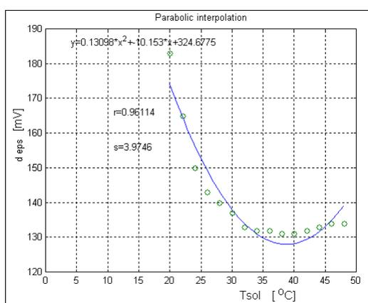
Fig. 10. The variation of the potential difference  $d_{eps}$  [mV] depending on the temperature of the NaCl solution, for a concentration of 9%.
