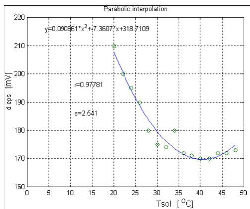
Fig. 5. The variation of the potential difference  $d_{eps}$  [mV] depending on the temperature of the NaCl solution, for a concentration of 4%.
