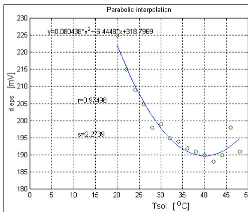
Fig. 4. The variation of the potential difference  $d_{eps}$  [mV] depending on the temperature of the NaCl solution, for a concentration of 3%.
