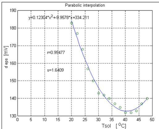
Fig. 12. The variation of the potential difference deps [mV] depending on the temperature of the NaCl solution, for a concentration of 11%.
