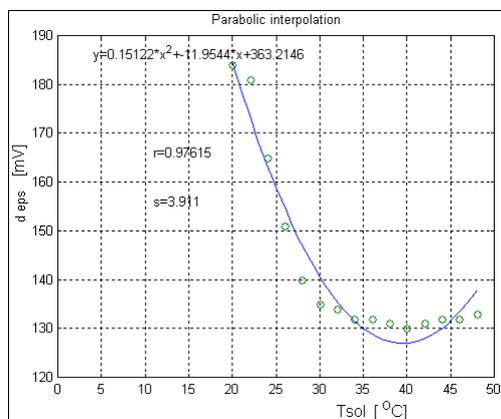
Fig. 9. The variation of the potential difference  $d_{eps}$  [mV] depending on the temperature of the NaCl solution, for a concentration of 8%.
