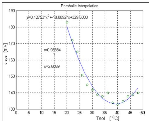
Fig. 15. The variation of the potential difference deps [mV] depending on the temperature of the NaCl solution, for a concentration of 14%.
