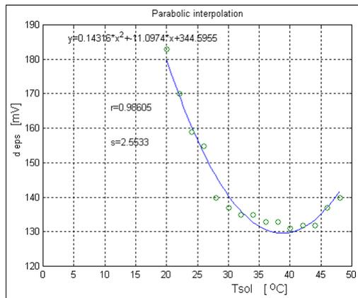
Fig. 14. The variation of the potential difference deps [mV] depending on the temperature of the NaCl solution, for a concentration of 13%.
