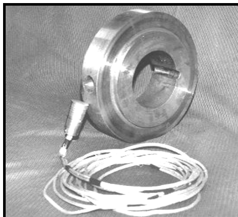
Figure 4. Thermo-coupled pin assembled and prepared for installation in the ring sample
