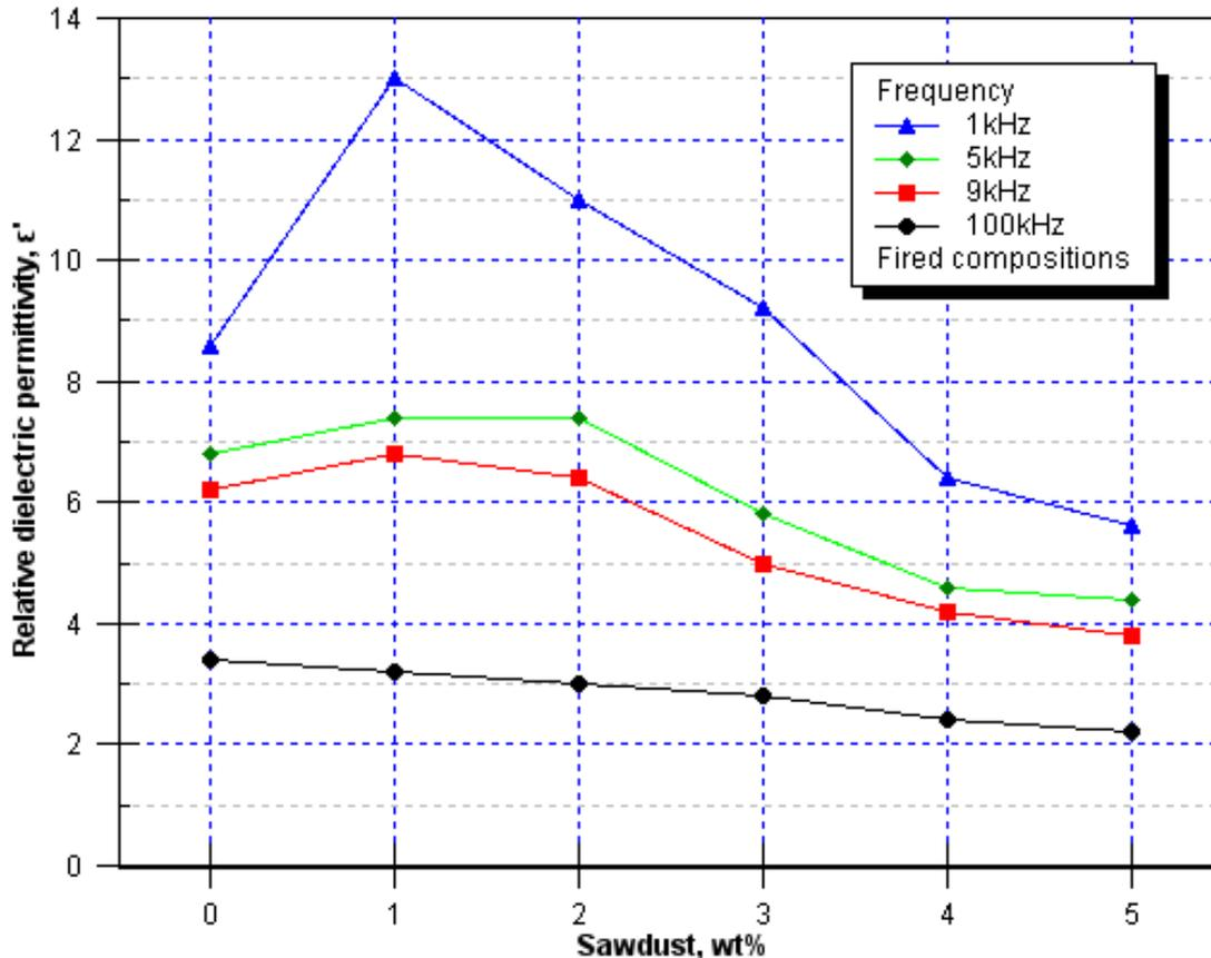
FIGURE 6. Relative dielectric permittivity of fired clay compositions as function of original sawdust concentrations
