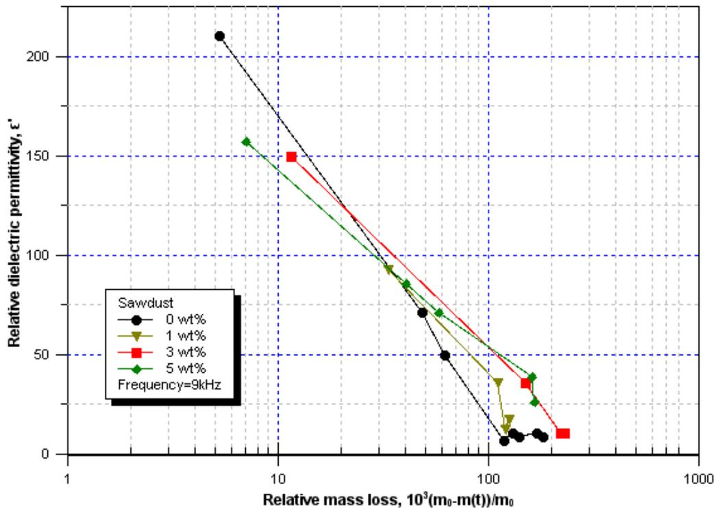
FIGURE 3. Changing the dielectric properties of different sawdust added samples during dehydration, measured at 9 kHz
