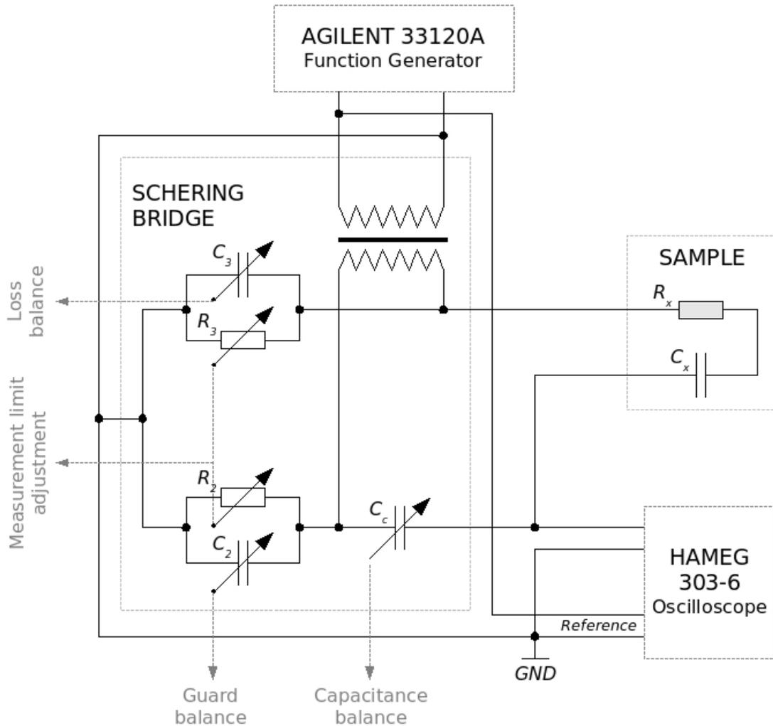
FIGURE 2. Schering bridge: Set up for dielectric measurements
