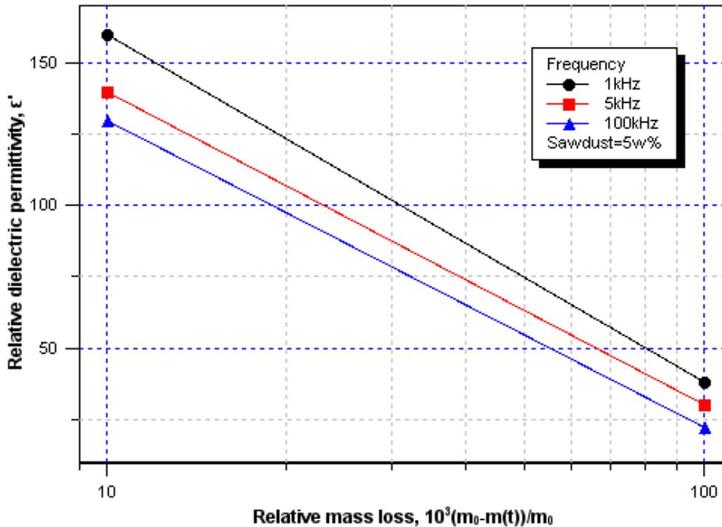
FIGURE 4. Changing the dielectric properties measured at different excitation frequencies during dehydration, sawdust content 5w%
