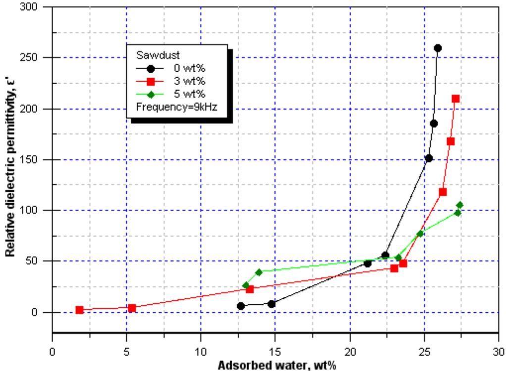
FIGURE 5. Relative dielectric permittivity as function of adsorbed water content measured at 9 kHz
