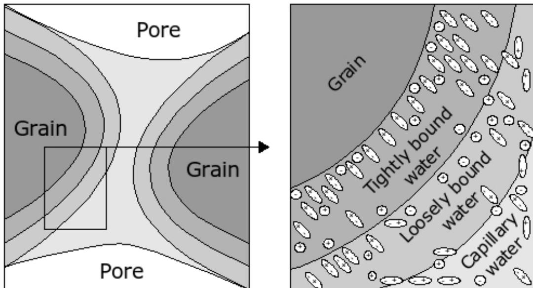
FIGURE 1. Structure of water found in clays [3]
